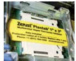
1" x 3" Plastab in an electronics enclosure.
